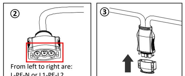
**Step 6.** Install a Bus Cable End Cap at the end of AC bus cable
