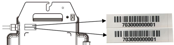
**NOTE:** ①.The layout of the microinverters' serial numbers installation map is only suitable for typical installation.
