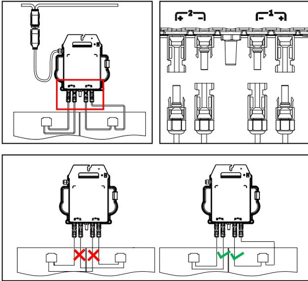
**NOTE:** When plugging in the DC cables, the microinverter should immediately blink red one time and green ten times. This will happen as soon as the DC cables are plugged in and will show that the microinverter is functioning correctly. This entire check function will start and end within 10 seconds of plugging in the unit, so pay careful attention to these lights when connecting the DC cables.
