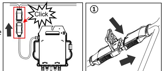
① **Best Practice:** Use the Bus Cable Unlock Tool of AC Bus to disconnect the connectors.
